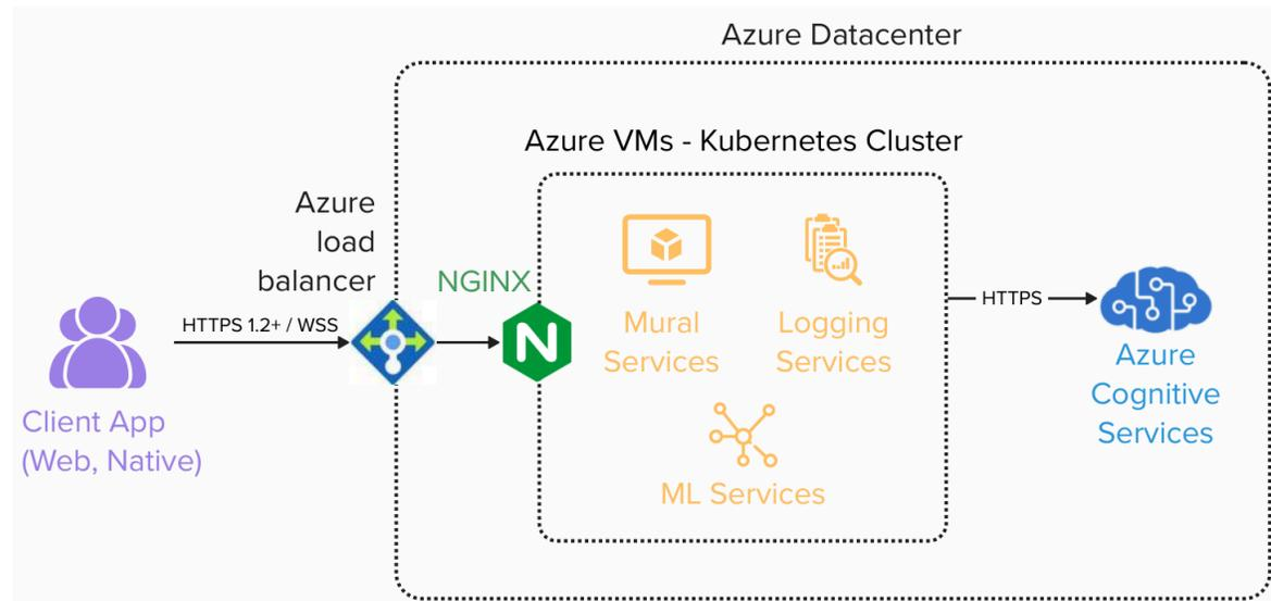
When an authenticated client performs an operation involving AI, our Mural Services check the credentials and make sure the client's permissions are right for accessing and modifying the objects, respecting tenancy and geo-location.
